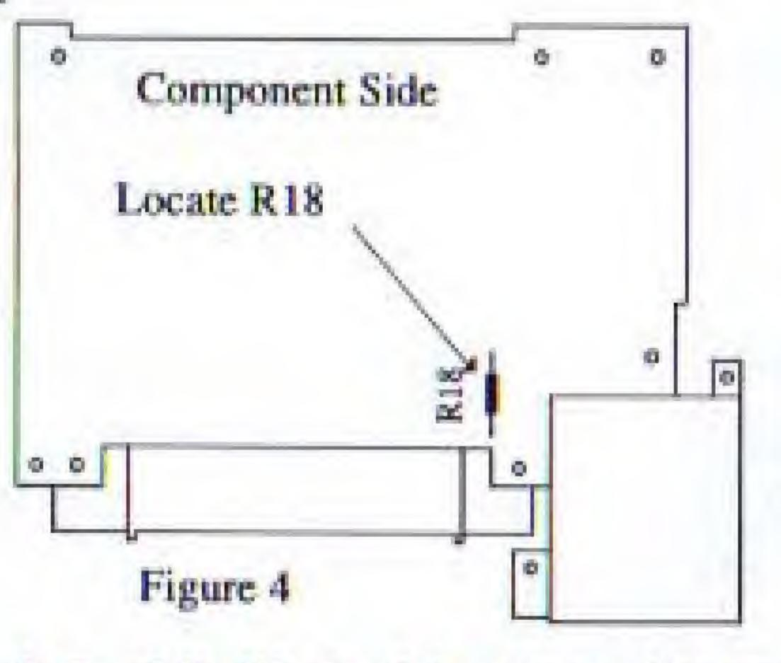
4. Carefully lift circuit board out of bottom and with all wires still attached turn board over. Be sure board is a Rev 11. This will be verified by the presence of R18 as indicated in Figure 4. If R18 is not present do not proceed! Call 1-800-HOT-4-AVE for assistance.
